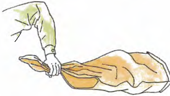
Figure 12A: Sandbag filled 1/4 to 1/3 full
